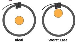
The position of the conductor inside the coil will affect the accuracy. Deviation from the centre will at worst cause a maximum of 1% deviation when the conductor is placed near the cap of the coil.
